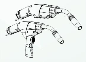
All Push-Pull torches are delivered with an extra handle for getting a pistol grip. Use the torch without the handle when welding in narrow passages.
